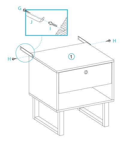
Insert the drawer as shown, ensuring it slides smoothly and easily along the rails. Once assembled lift the furniture into place, do not drag.
