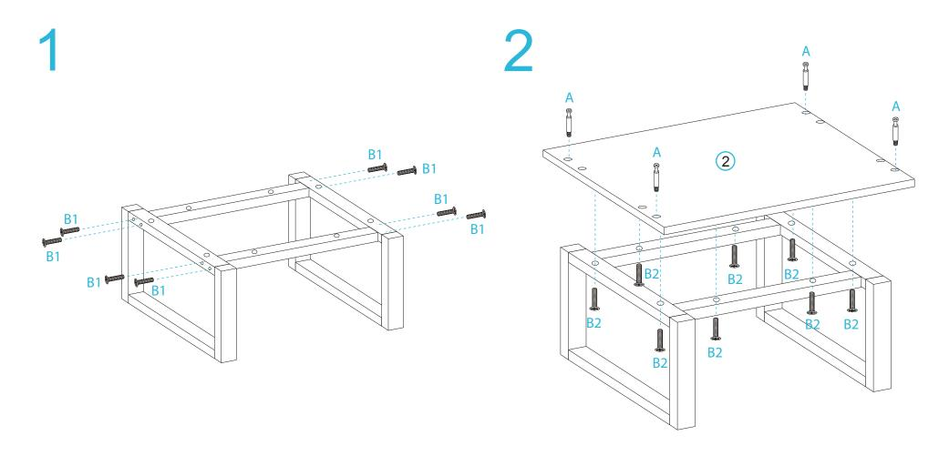
Attach the leg panels together as shown using 8x 50mm screws (B1). Tighten with a screwdriver.
