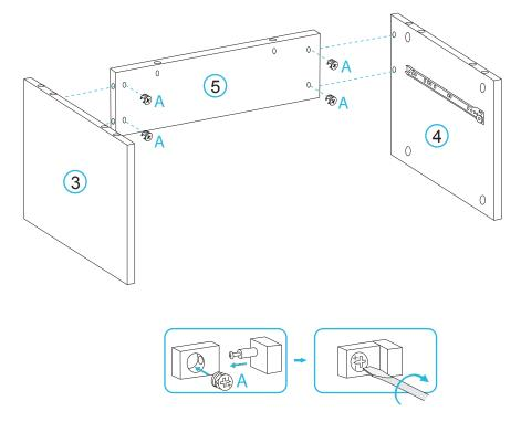
Insert 2x bolts (A) and attach 1x slide rail (E1) to panel [3] using 2x 12mm screws (C). Insert 2x bolts (A) and attach 1x slide rail (E3) to panel [4] using 2x 12mm screws (C). Tighten with a screwdriver.
